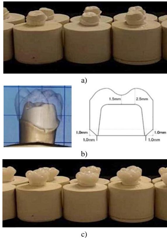
**Figure 3.** Resin test blocks; a) resin test blocks with embedded duplicate abutment teeth, b) digital scan and design of the tested PICN hybrid ceramic crown, and c) resin test blocks with cemented crowns.
