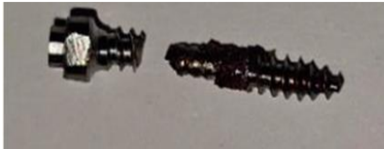
Figure 2. Results for the mini-implant under 2 N loading at 30°: (a) Total deformations; (b) von Mises equivalent stresses; (c) Equivalent strains; (d) The mini-implant was fractured after removal precisely in the area where the FEM analysis indicated the maximum von Mises stress.
