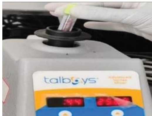
Figure 6. Vortexing of disinfected implants in 10 ml of thioglycollate broth for 60 s
