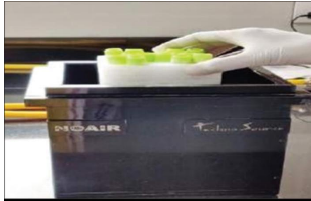
Figure 4. Vials containing Porphyromonas gingivalis contaminated implants placed in an anaerobic jar
